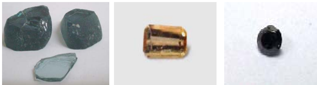
FIG. 3 (Left) Topaz from Rondônia, RO, Brazil; (Centre) spodumene from the east of Minas Gerais, MG, Brazil and (Right) diamond from Minas Gerais, MG, Brazil after neutron irradiation with dose of 10^{18} , 10^{17} and 10^{18} neutrons/cm 2 .
